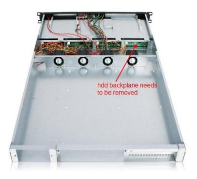
4. Slide the 3.5" tray back to the chassis and connect the power and data cables.
