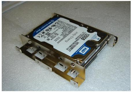
2. Take out the 3.5" tray from E1M4 and mount the RP-HDD2.5 onto the tray. (We need to use flat head screws, so that the tray can slide back into the chassis)
